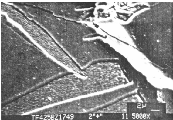
Figure 3 – Origin of the double on the twin border with small degree of coherency
